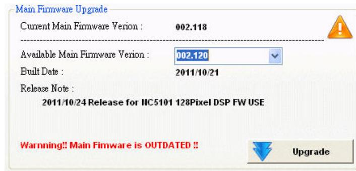
3. Always update the machine if a warning triangle is displayed for a component.
