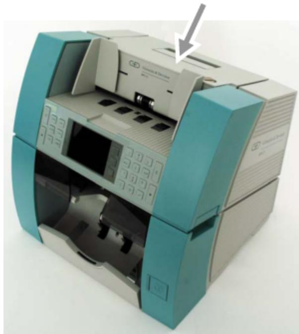
4. Press the upper module downward on the cover (arrow).
